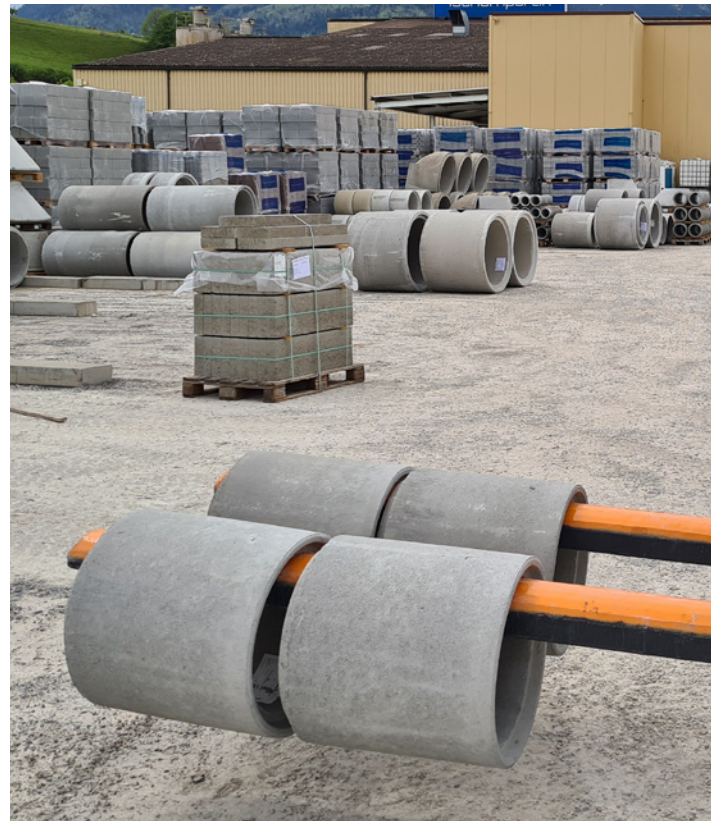
CROC Spray coating: Concrete elements do not slip off the forks
